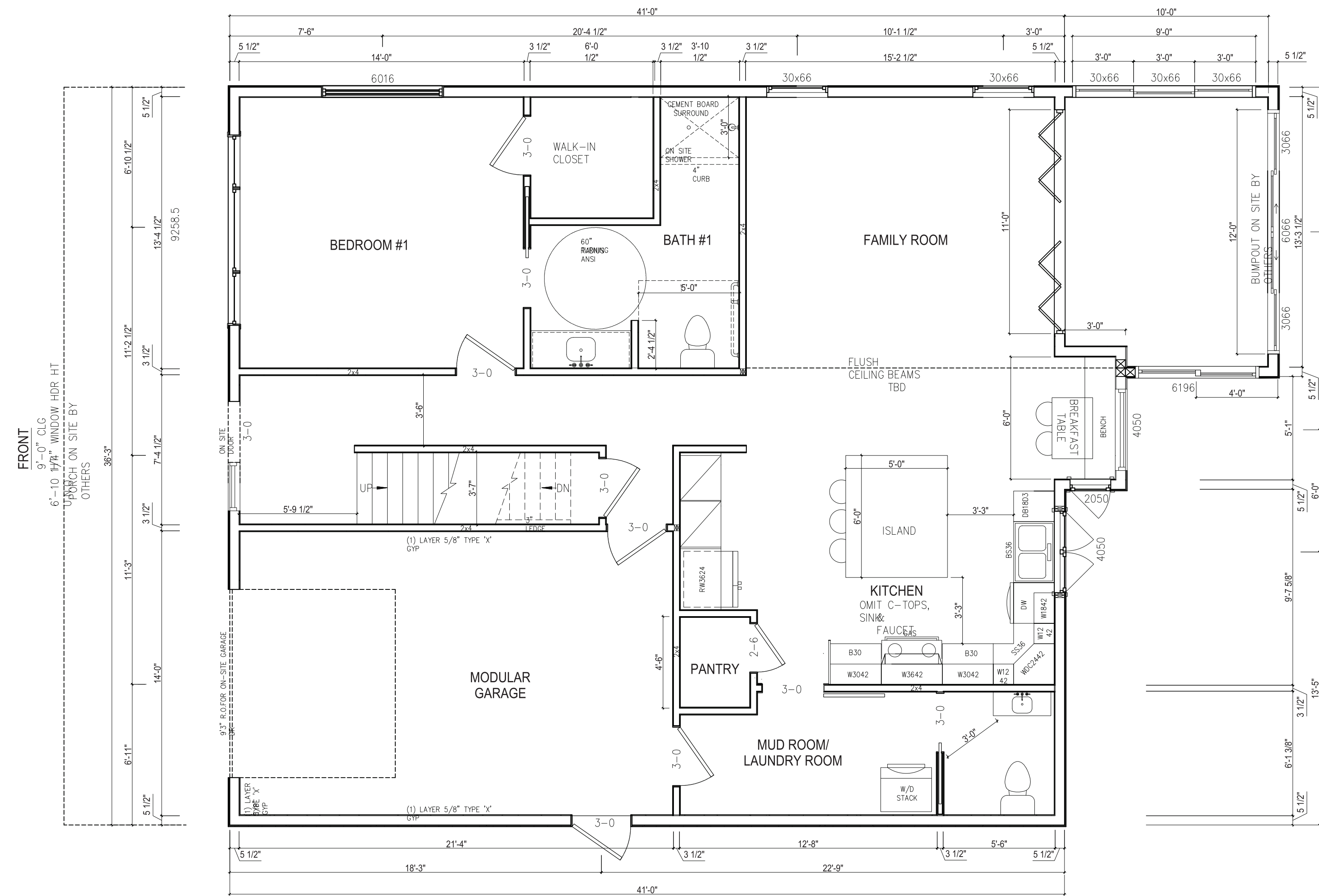
FIRST FLOOR PLAN SCALE: 1/4" = 1'-0"
