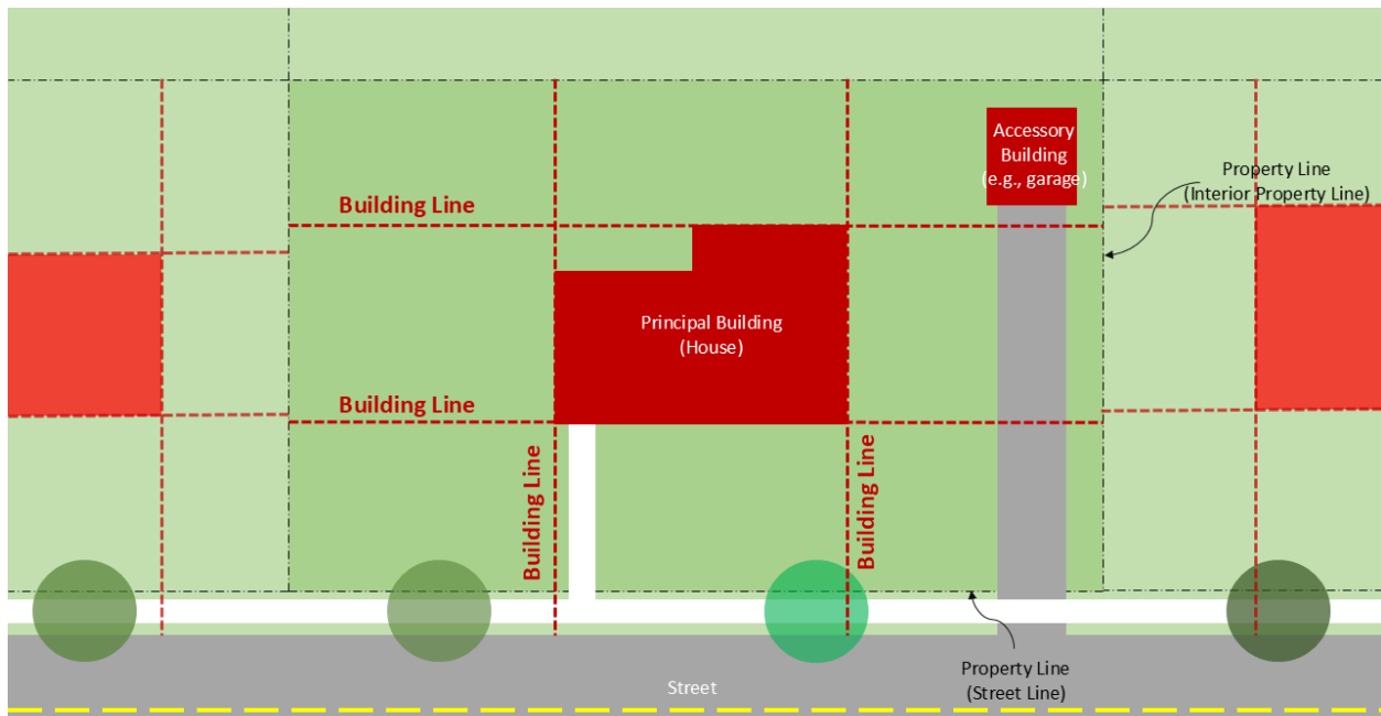
Fig. 3.1 Building Lines - for illustrative purposes only -
