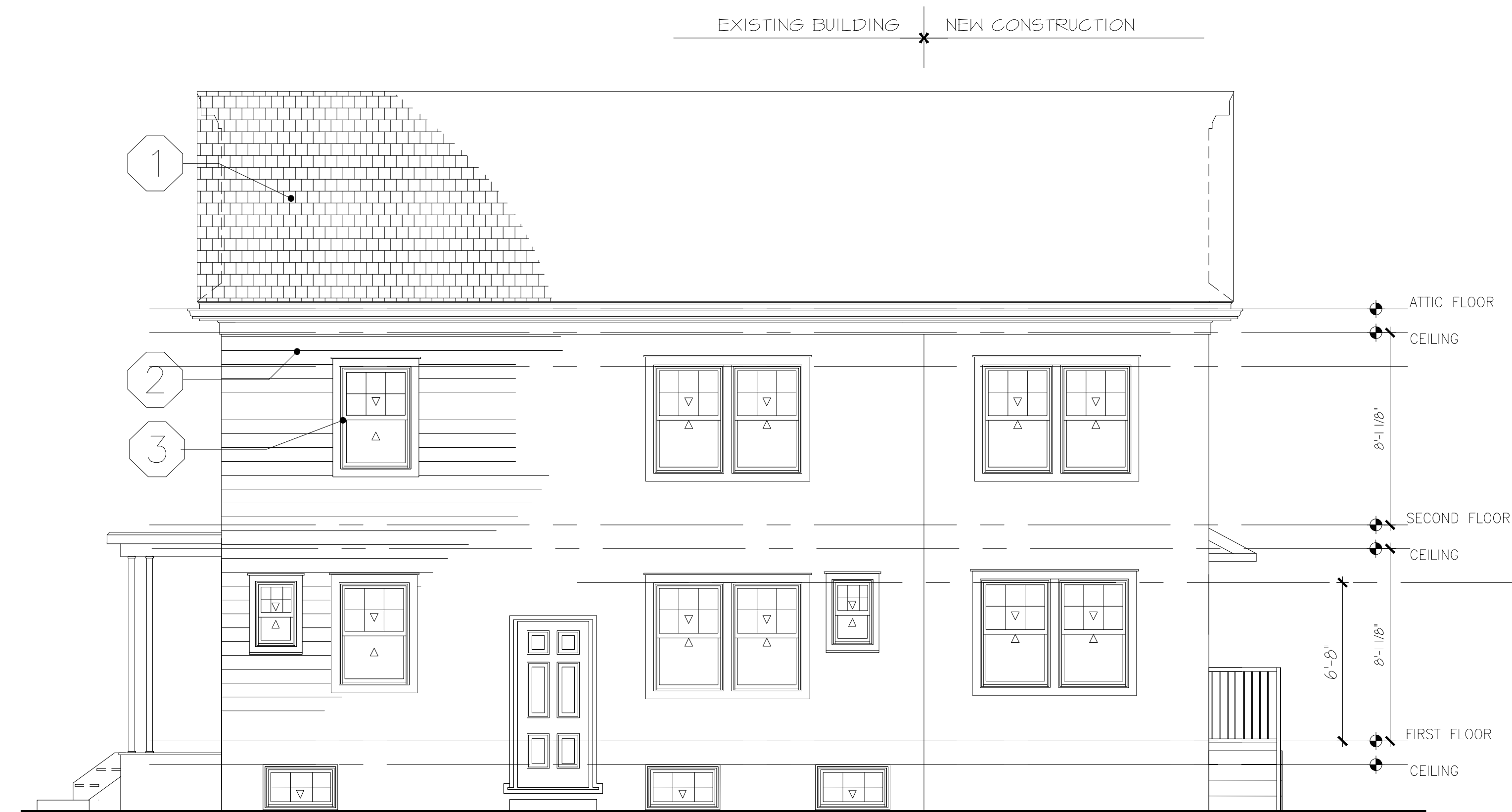
6 PROPOSED WEST ELEVATION 1/4"=1'-0"
