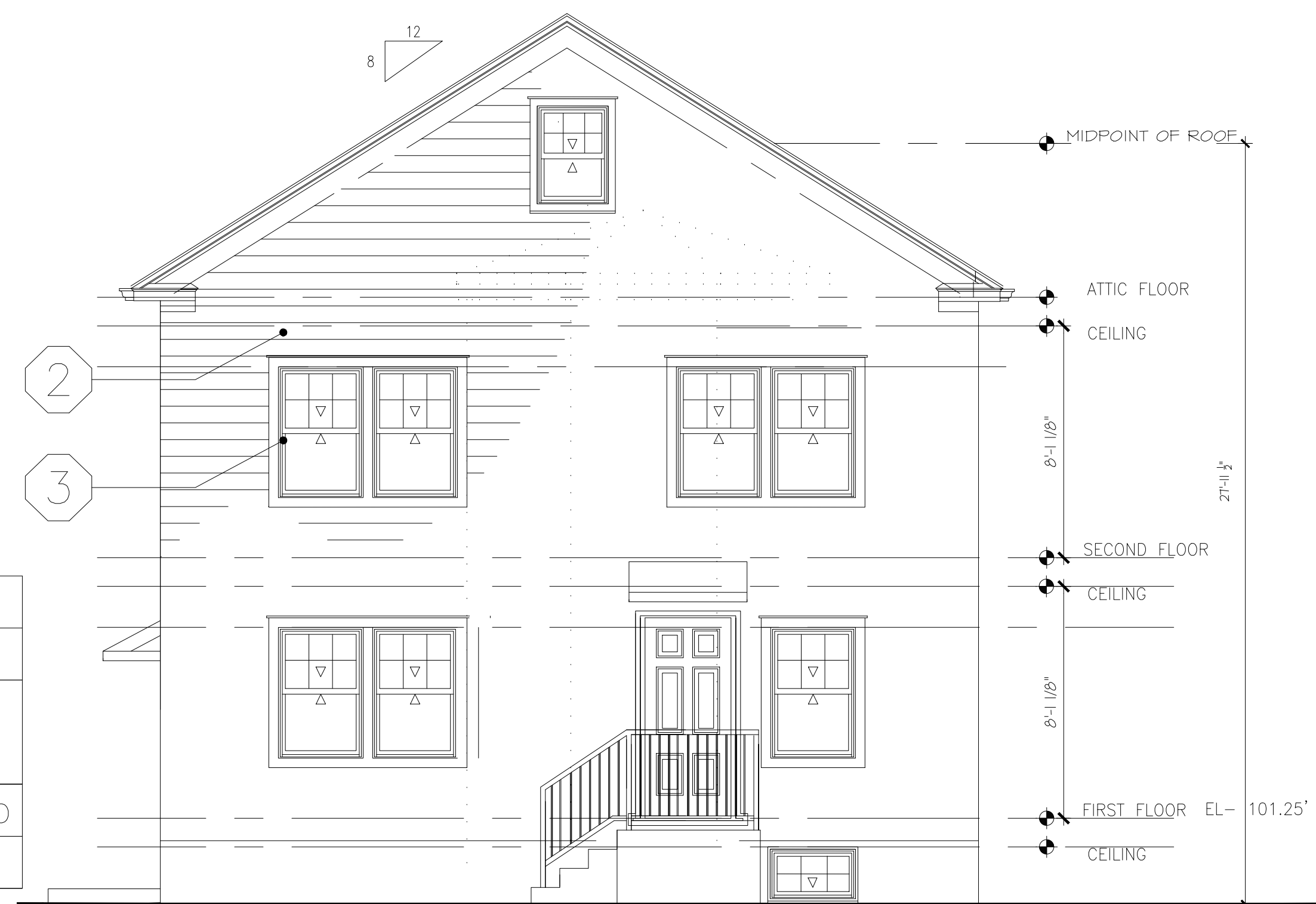
5 PROPOSED SOUTH ELEVATION 1/4"=1'-0"
